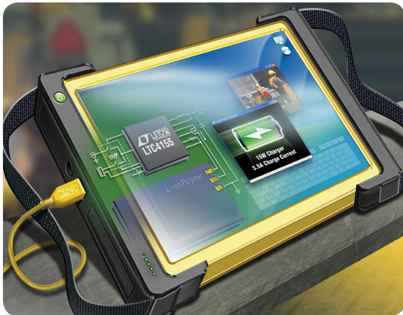
The LTC4155 is a monolithic switching battery charger that efficiently delivers 3.5A charge current in a compact PCB footprint. See page 13.
